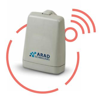
The Dialog3G<sup>™</sup> Universal unit is suited for different input connection types such as the "Single switch type", where up to four independent meters can be connected to one 3G Universal unit. Each input has its own reading/ programming parameters. "Single input type" for PD meters with a 3 wire pulse output, or serial communication for individual multiphase electricity meters. Controlled I/O Universal unit for MagneLatch type Valves
