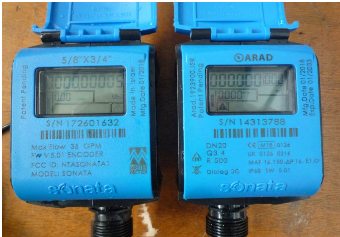
Photograph 6.2.3 The EUT inspection after immersion test
