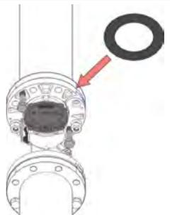
Insert a gasket between the floating flange and the pipeline flange
